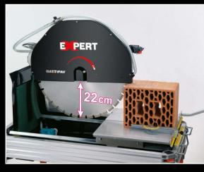
The cutting position with sliding carriage.
