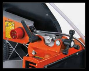
Adjustament system of the cutting height with an hand wheel and relevant locking lever. Possibility to make cuts with **2 RUNS** (max depth 340 mm).
