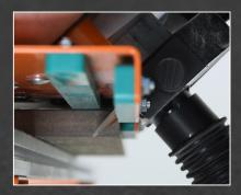
Adjustable bevel depth, with maximum cutting height of 21 mm, disc cover with dust extraction.
