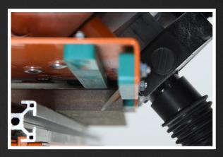
Adjustable in depth, with maximum cutting height of 21 mm, disc cover with dust extraction.
