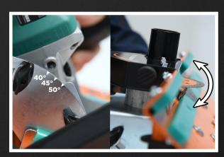
Adjustable cut for inclinations from 40° to 50°.
