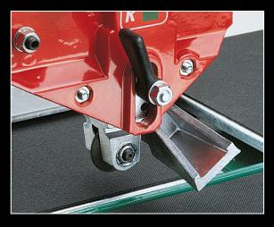
**CUTTING WHEEL**Tungsten carbide cutting wheel of big dimension: Ø 22 mm.
